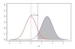
▶ When *c* is larger, the test's size becomes smaller and so does the power.
